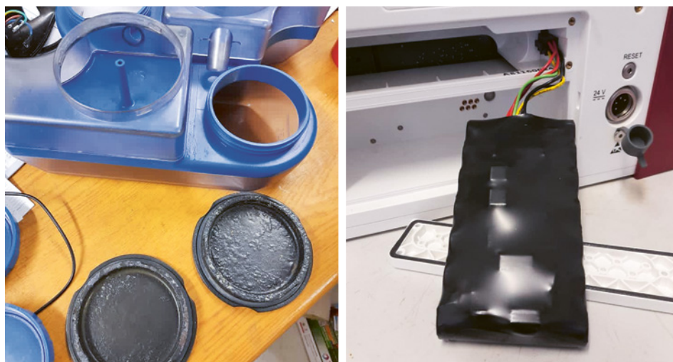
Fig. 9. Proper equipment maintenance will be crucial: damaged humidifier chambers of MTTs Dolphin® CPAP machines (left); malfunctioning internal battery of the EVE® neo ventilator (right).
